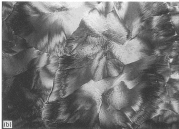
Figure 1 (a, b) Micrographs of Epikote 1001/phthalic anhydride system obtained from acetone solution after drying at room temperature.
