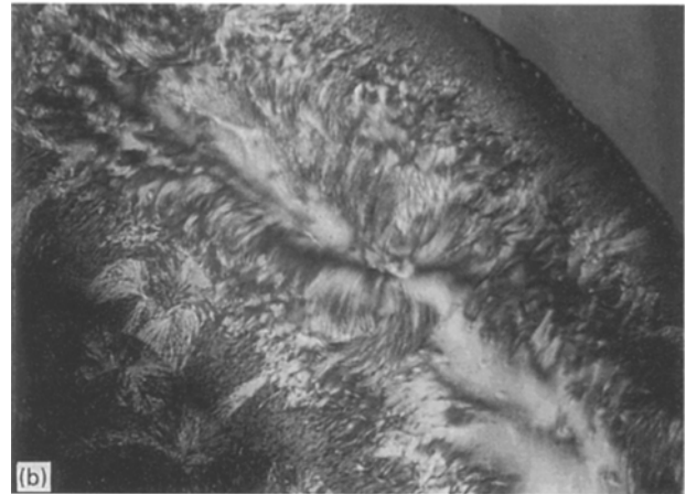
Figure 3 (a, b) Micrographs of Epikote 1001/phthalic anhydride system obtained from acetone solution after drying at 80^\circ\text{C} .
