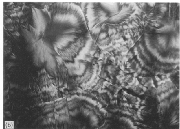
Figure 2 (a, b) Micrographs of Epikote 1001/phthalic anhydride system obtained from acetone solution after drying at 45^\circ\text{C} .
