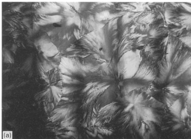
Figure 2 (a, b) Micrographs of Epikote 1001/phthalic anhydride system obtained from acetone solution after drying at 45^\circ\text{C} .
